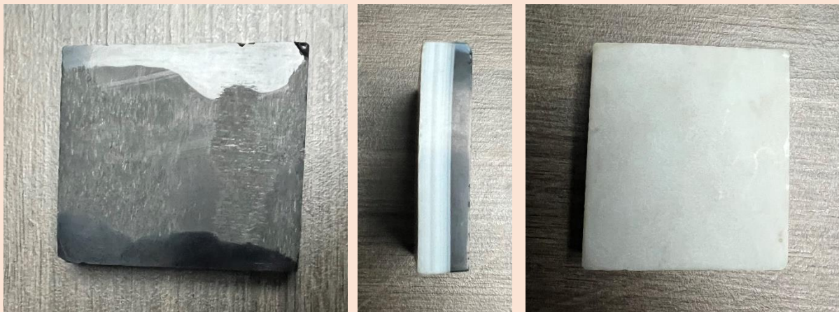
The roughly polished agate slab, colored black in the broad lower layer, as the starting material. The middle picture shows up to eight layers of chalcidony in slightly different colors.
