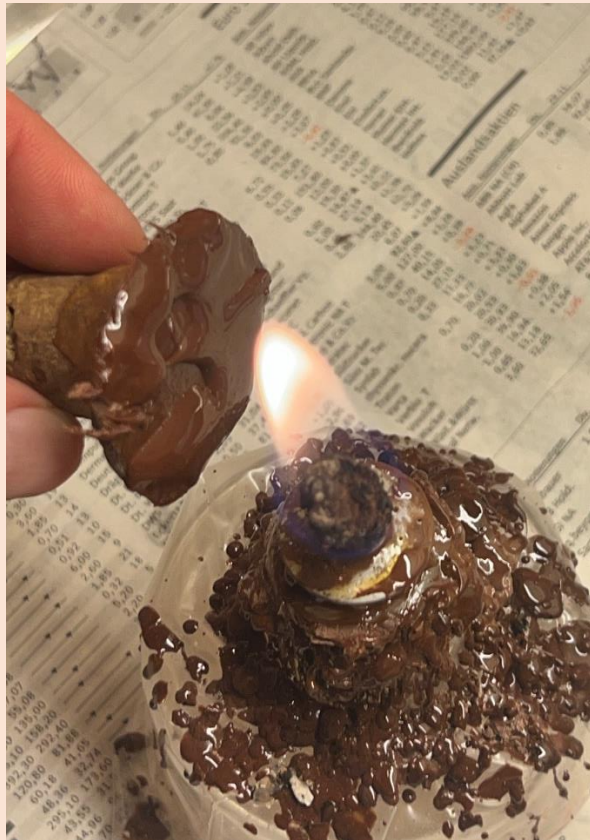
Further preparation and cementing of the stone with sealing wax on a fixing rod.
